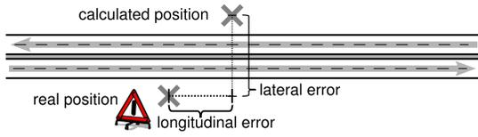
Figure 2. Longitudinal and lateral error in the position calculation.
