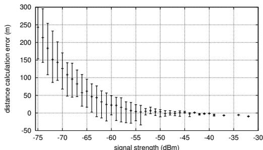
Figure 5. Distance computation-error using the Free-Space-Model.
