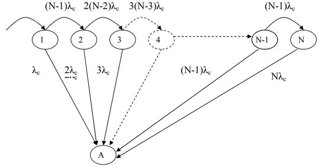
Fig. 1. Transition diagram of Markov chain for finite message dissemination
